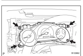
**32. REMOVE COMBINATION METER ASSEMBLY** (a) Remove the 4 screws.
