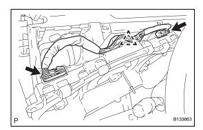
(b) Disconnect the 2 connectors and clamp and remove the combination meter.
